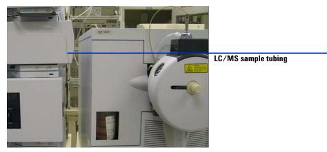
Figure 19 LC/MS sample tubing connected to LC/MS inlet filter
